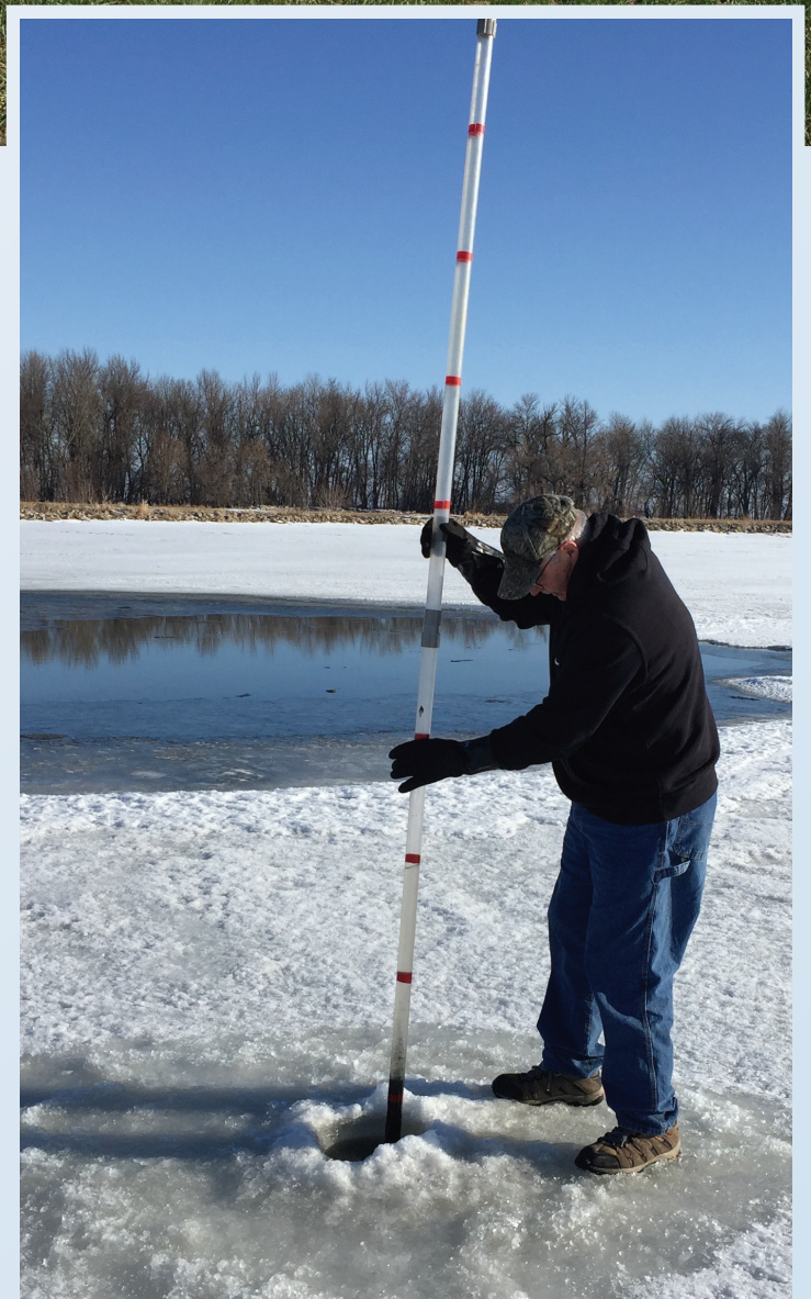
Les Sigette, NDRWSA wastewater technical, using the sludge judge to determine sludge depth.
